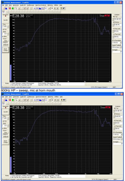
Rank on 340 horn – 400Hz HP – sweep, mic at horn mouth
