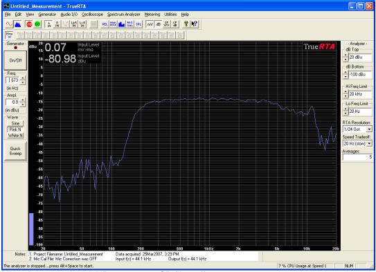
Mic at horn mouth, 160HP cross over, CD filter off
