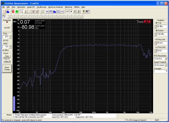
Mic at horn mouth, 160HP cross over, CD filter on
